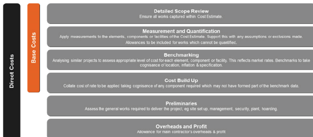
Figure 19 Approach to Cost Estimating, Direct Costs
